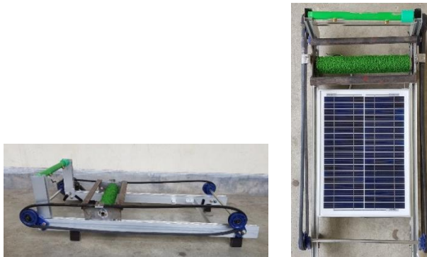
Fig. 7: Fabricated Model of Single Axis Cleaning System
